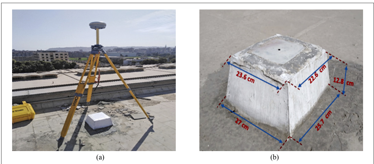
Figure 3: Field points sites a) “TADN” field station occupied with the Trimble geodetic GNSS receiver b) “MECH” Station shape and size.
