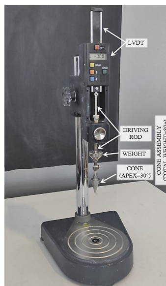
Figure 1: Fall cone device with 30° cone apex and 80g cone assembly weight according to BS 1377-2, 1990
