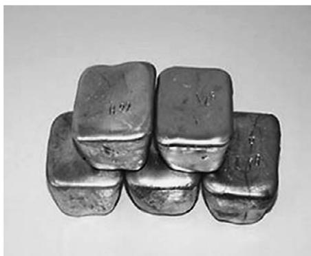
Figure 3 Polished rare earth metal ingot
