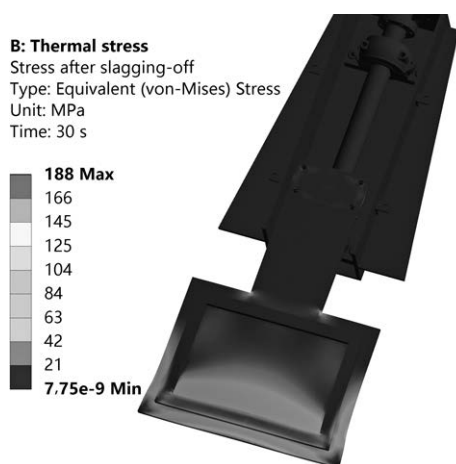
Figure 8 Thermal stress of robotic arm
