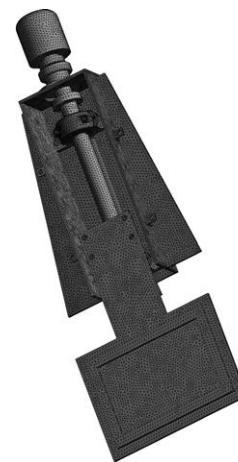
Figure 1 Finite element model of slagging-off robot arm
