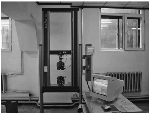
Figure 1 High speed material testing machine
