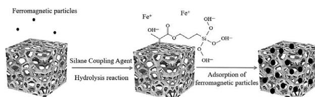
**Figure 1** Principles of magnetorheological sponge synthesis
