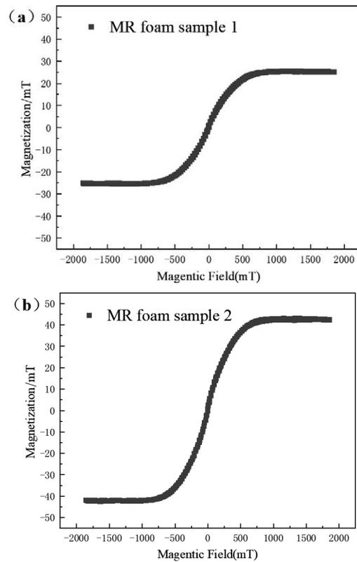
Figure 3 Magnetization curve
