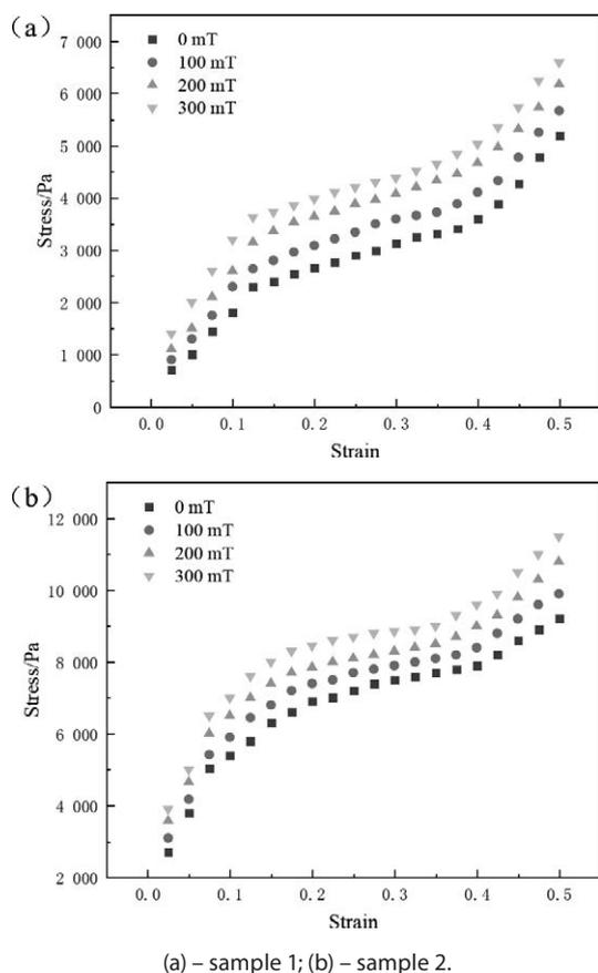
**Figure 5** Stress-strain relationship of MR sponge under different magnetic fields
