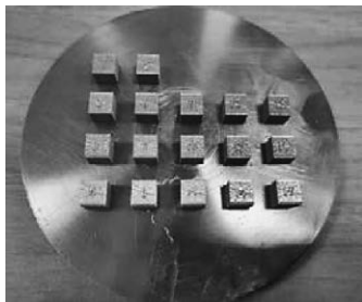
Figure 2 Printing results of block specimens
