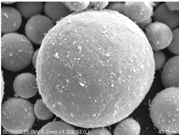
**Figure 6** Powder after ball milling
