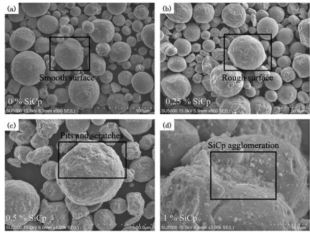
**Figure 4** SEM images of mixed powders with different SiCp contents
