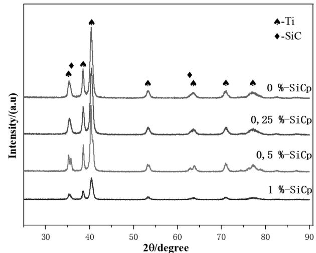
**Figure 5** XRD patterns of mixed powders with different SiCp contents
