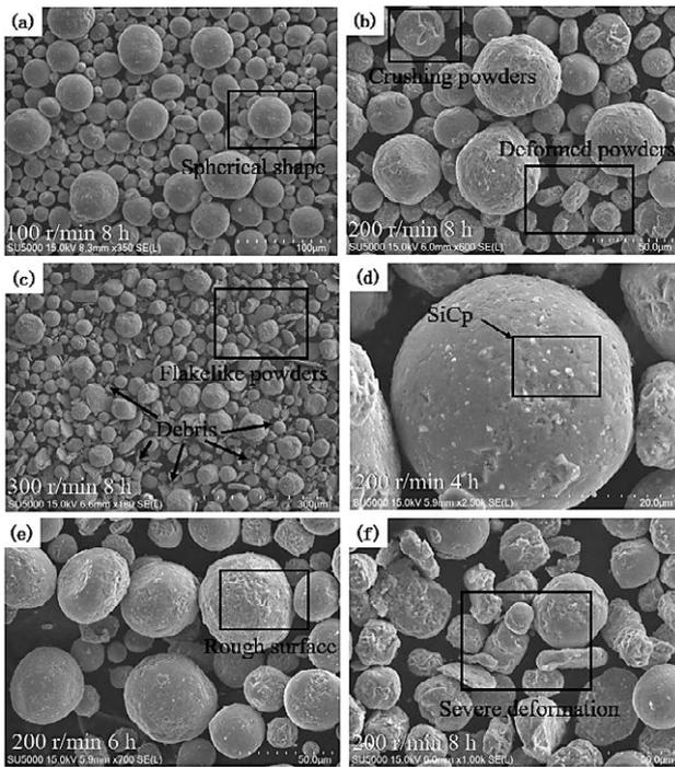
**Figure 2** SEM of the mixed powders at different milling parameter.
