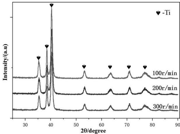
**Figure 3** X-ray Diffraction(XRD) patterns of mixed powders with different milling speeds
