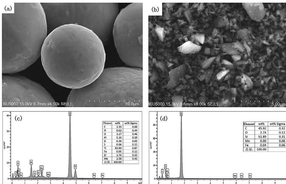
**Figure 1** Scanning electron microscopy microstructure (SEM): (a) TC11, (b) SiC; Energy Dispersive spectrometer analysis (EDS): (c) TC11, (d) SiC
