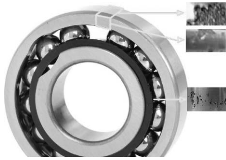
Figure 7 Examples of bearing failures
