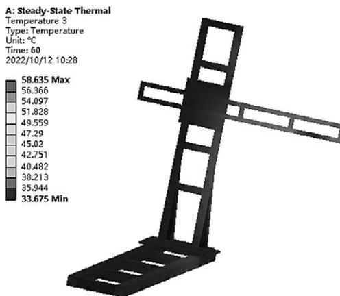
Figure 2 Temperature of Rare earth electrolytic robot
