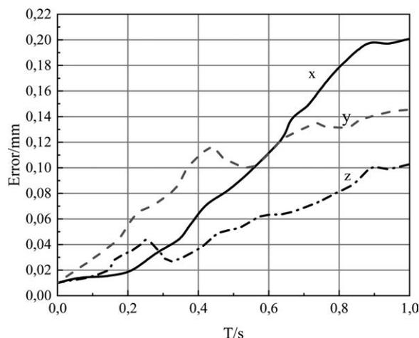
Figure 6 Length dimension error curve of connecting rod of walking mechanism
