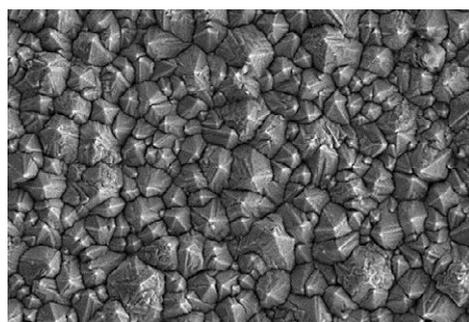
**Figure 5** SEM image of cobalt coating
