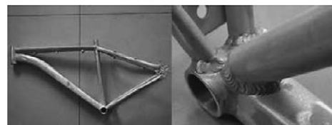
Figure 1 6061-T6 aluminum alloy bicycle frame
