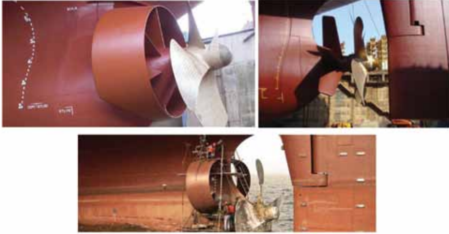
Figure 2. Mewis duct (top left), pre-swirl stator (top right), and Schneekluth duct (bottom) Slika 2. Mewis vod (gore lijevo), predvrtložni stator (gore desno), Schneekluth vod (dolje)
