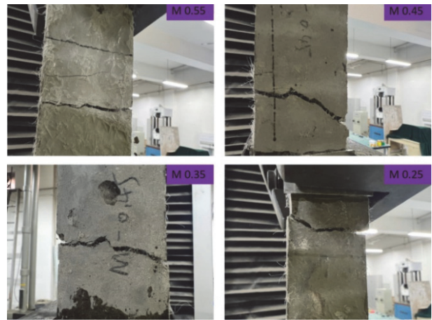
Figure 7 Crack morphology of specimen in a direct tension test
