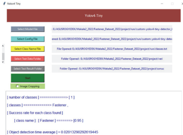
Figure 5 GUI design for testing the YOLOv4-Tiny model
