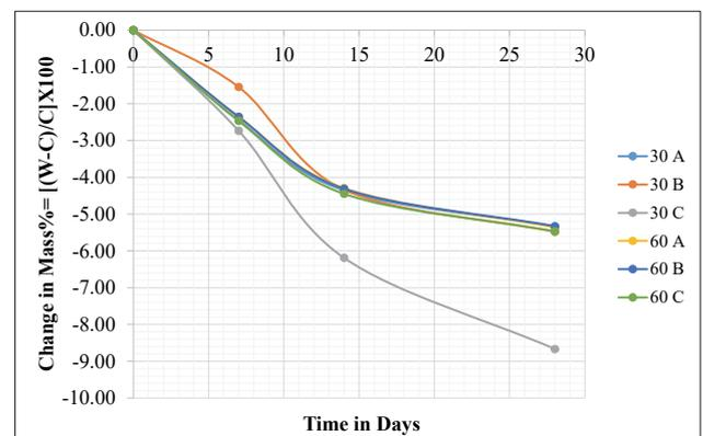
Figure 11 Acid test 30% replacement of bentonite mix SCC
