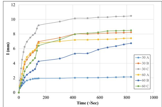
Figure 4 Sorptivity of different strength control mix SCC
