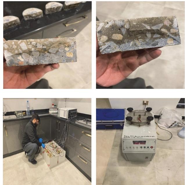
**Figure 2** Migration coefficient preconditioning and testing
