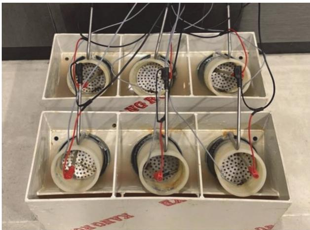
**Figure 1** Non-steady state chloride migration test arrangement
