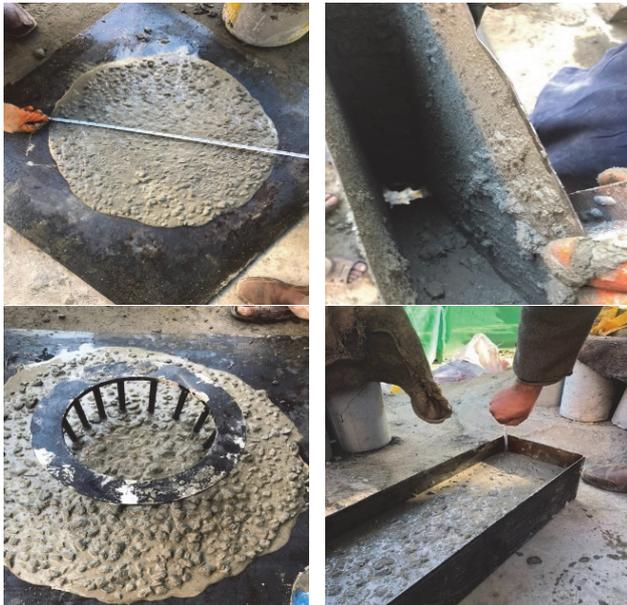
Figure 3 Various tests for fresh properties of SCC
