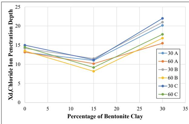
Figure 8 Chloride ion penetration depth with varying level of BC
