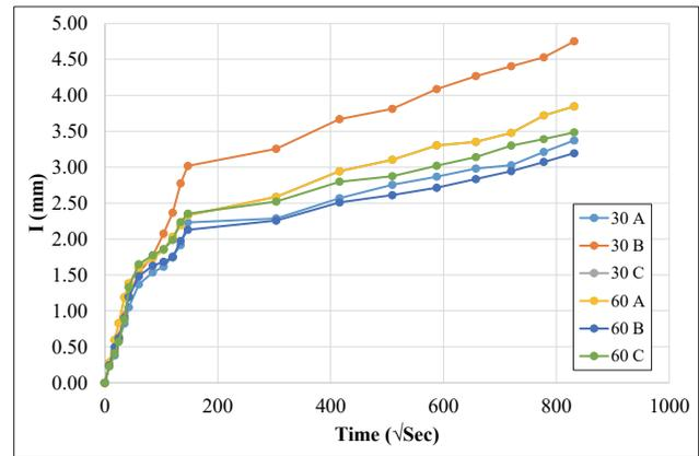
Figure 5 Sorptivity of different strength 15% replacement mix SCC
