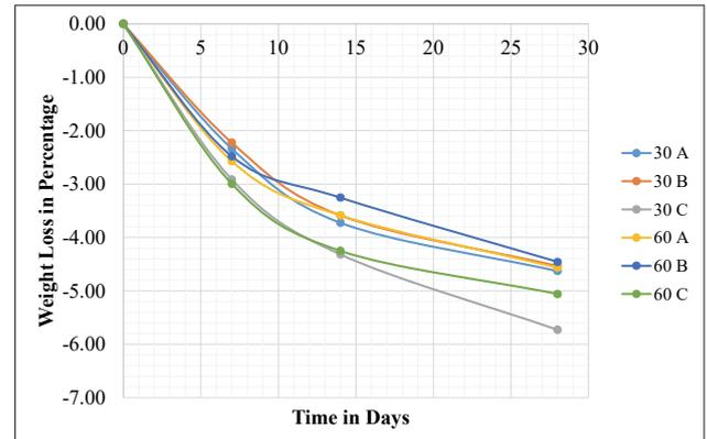
Figure 9 Acid test results of different strength control mix SCC
