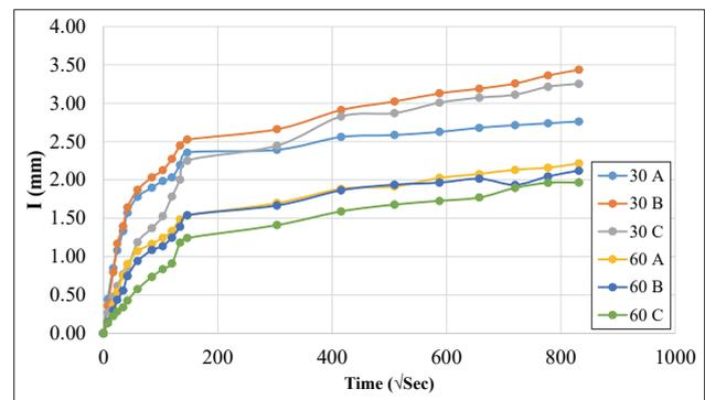
Figure 6 Sorptivity of different strength 30% replacement mix SCC
