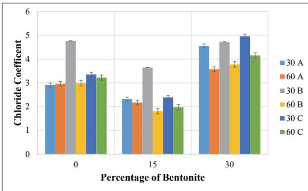
Figure 7 Chloride migration coefficient with varying level of BC
