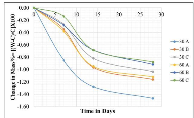
Figure 10 Acid test 15% replacement of bentonite mix SCC
