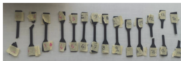
Figure 7 The test sample after the static tensile test
