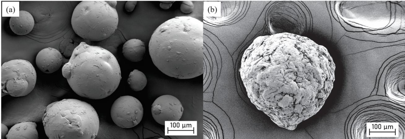
Fig. 2 – FE-SEM images of PE microplastics (a) and cellulose particles (b)
