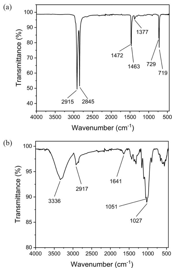
Fig. 1 – FTIR spectrum of PE microbeads (a) and cellulose particles (b).
