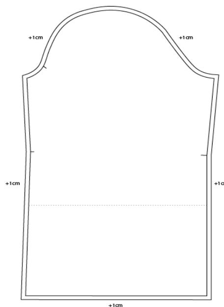
Fig.16 Sleeve pattern part with seam allowances [27]
