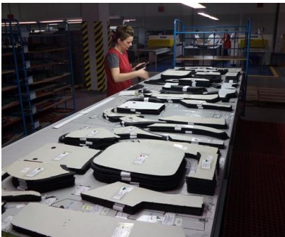
Fig.4 Sorting and checking of the seat cover parts after cutting
