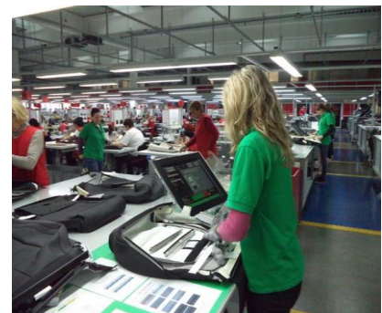
Fig.7 Final control after completion of the technological process of sewing car seat covers
