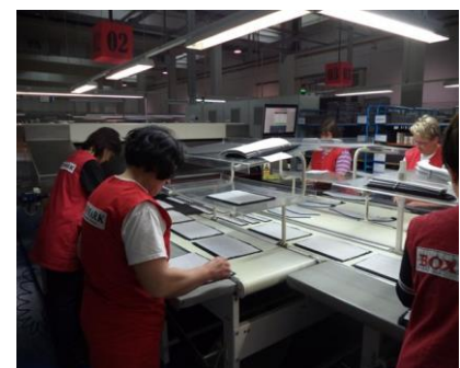
Fig.3 Placing the cover parts in the thermos-tunnel to activate the laminating adhesive
