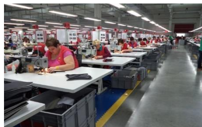
Fig.6 Production line in the technological process of sewing car seat covers
