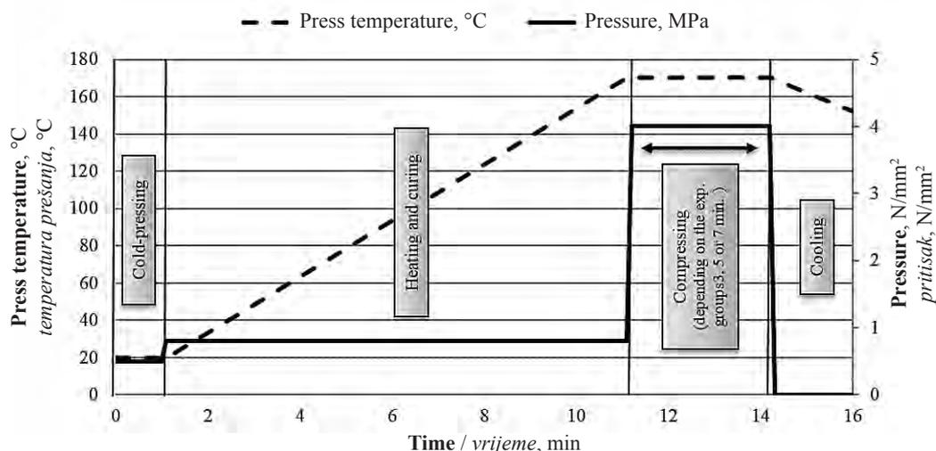
**Figure 1** Schedule of dLVL pressing process**Slika 1.** Raspored procesa prešanja ugušćene lamelirane drvene građe
