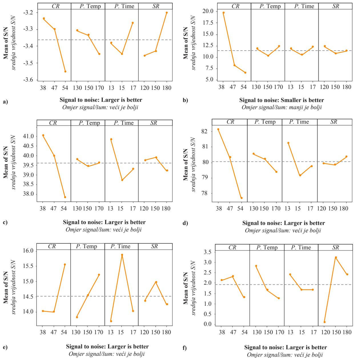
**Figure 2** Main effect plots for *S/N* of d (a), *SB* (b), *MOR* (c), *MOE* (d), *TSS* (e), and *TSPS* (f)
