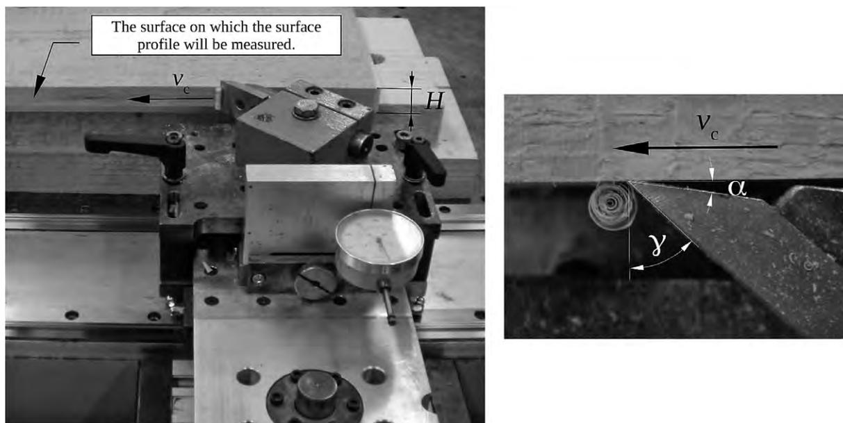
**Figure 1** Cutting of test specimens of solid oak wood (*Quercus robur* L.) with average cutting width  $H = 21$  mm in  $90^\circ - 0^\circ$  direction with cutter made from high-speed steel (HS), with rake angle  $\gamma = 50^\circ$ , clearance angle  $\alpha = 8^\circ$ , chip thickness  $h = 0.03$  mm and cutting speed  $v_c = 0.5$  m/s to obtain Type II - continuous chip
