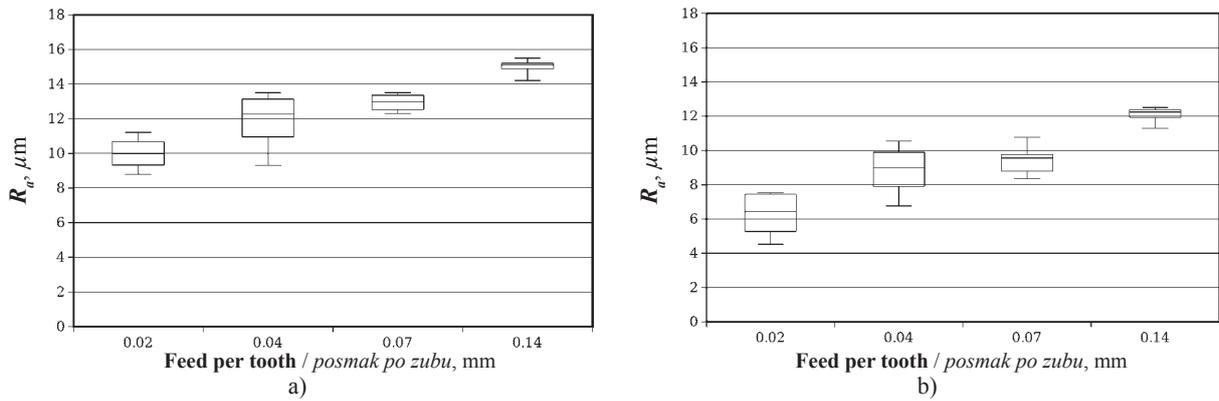
**Figure 6** Machined surface roughness expressed through parameter  $R_a$ : a) after sawing solid oak wood with different values of feed per tooth and b) for processing roughness signal, after filtering total roughness signal with filter based on FFT and threshold obtained in this research
