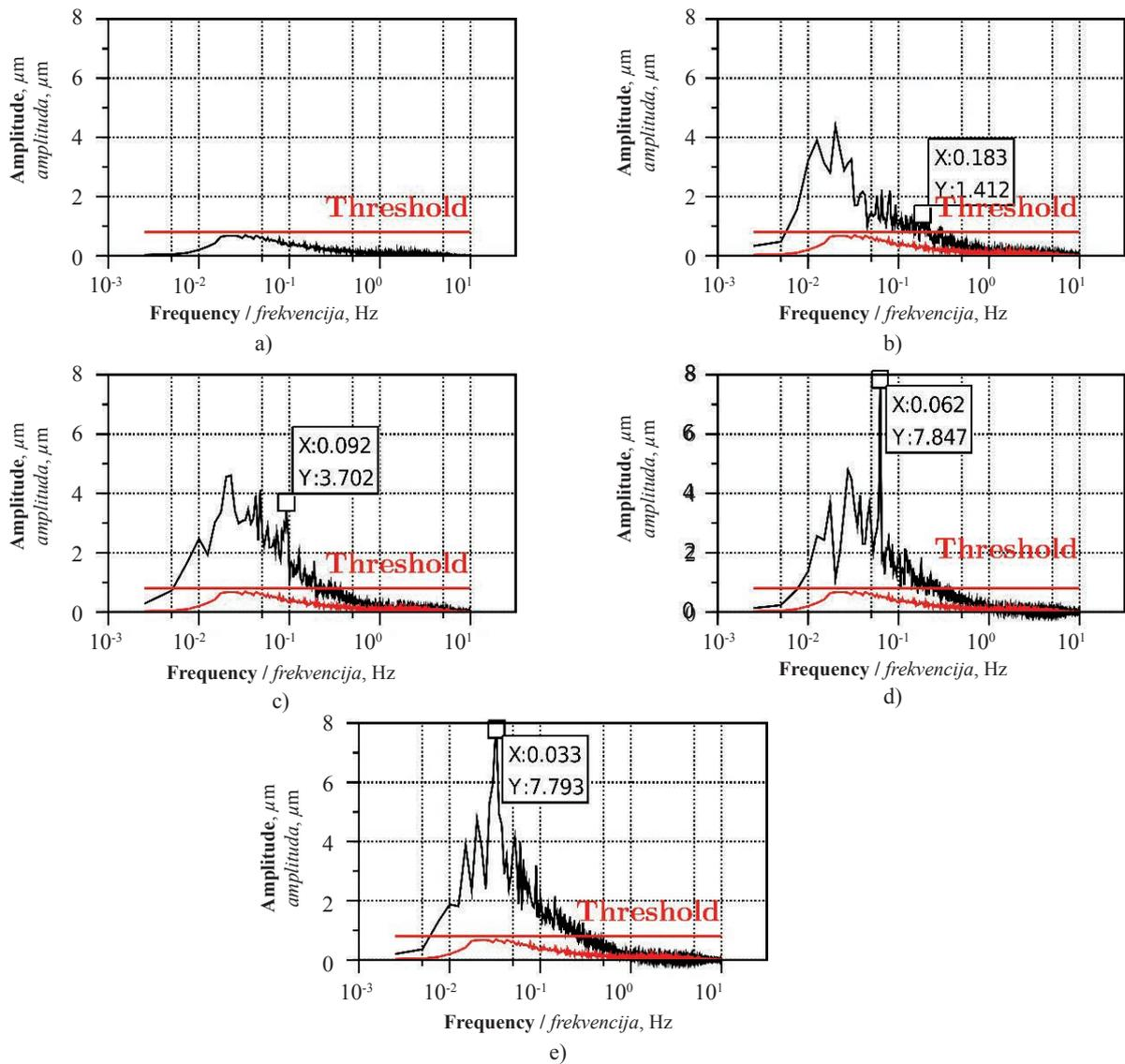
**Figure 7** Comparison of frequency spectra of averaged surface roughness profiles for: a) anatomical roughness, b) machined surface roughness after sawing with  $f_z = 0.02$  mm, c) machined surface roughness after sawing with  $f_z = 0.04$  mm, d) machined surface roughness after sawing with  $f_z = 0.07$  mm and e) machined surface roughness after sawing with  $f_z = 0.14$  mm
