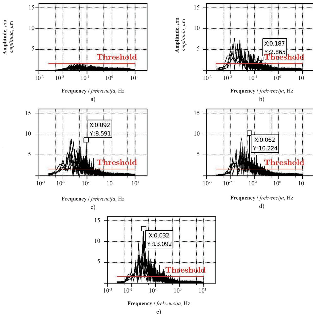
**Figure 5** Comparison of frequency spectra for samples of measured surface roughness profiles against objectively determined value of threshold for: a) anatomical roughness, b) machined surface roughness after sawing with  $f_z = 0.02$  mm, c) machined surface roughness after sawing with  $f_z = 0.04$  mm, d) machined surface roughness after sawing with  $f_z = 0.07$  mm and e) machined surface roughness after sawing with  $f_z = 0.14$  mm
