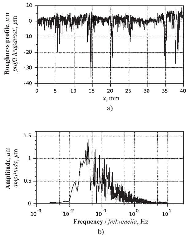
**Figure 3** Sample of a) anatomical surface roughness profile (R profile) measured on radial cross-section of solid oak wood (*Quercus robur* L.) and b) frequency analysis of that signal
