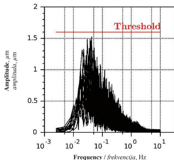
**Figure 4** Frequency spectra of measured anatomical surface roughness signals and threshold used for further signal processing of surface roughness signals obtained from measurements on machined surface after sawing with circular saw
