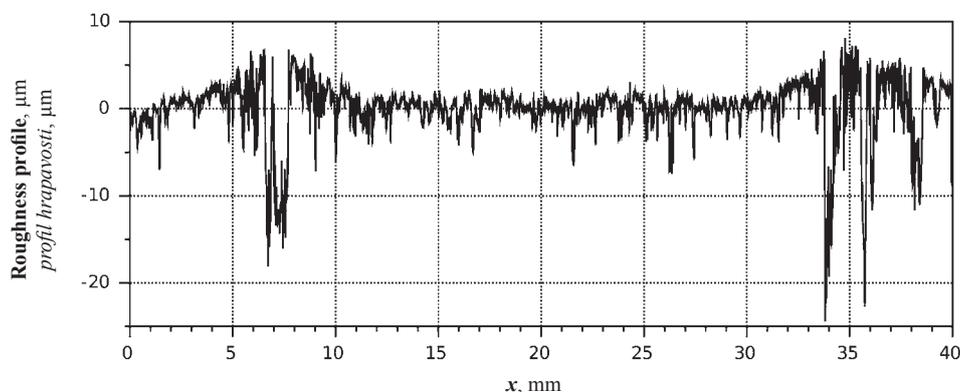
**Figure 2** Anatomical surface roughness profile (R profile) sample of radial cross-section of solid oak wood (*Quercus robur* L.) measured with surface roughness tester Mitutoyo SurfTest SJ-500, with the  $\lambda_s = 25 \mu\text{m}$ ,  $\lambda_c = 8 \text{ mm}$ , evaluation length  $40 \text{ mm}$ , stylus traversing speed  $v_s = 0.1 \text{ mm/s}$  and filtered with Gaussian filter
