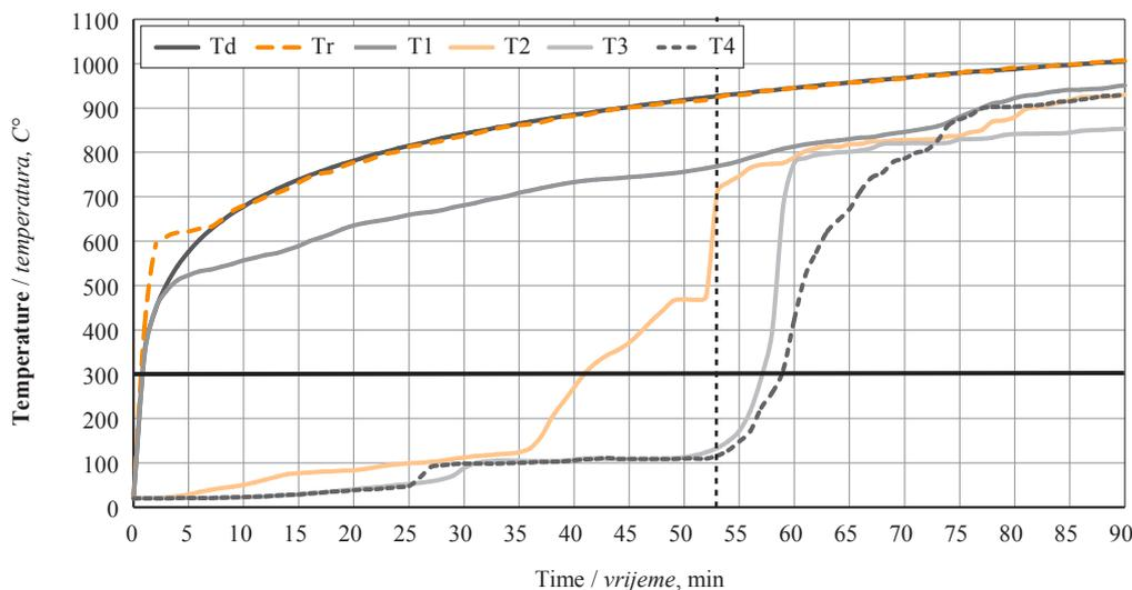
**Figure 8** Temperature trends of test specimen TS3 in thermocouples T1 to T3 depending on actually reached temperature  $T_r$  in fire furnace with marked significant time points,  $T_d$  is fire furnace reference temperature
