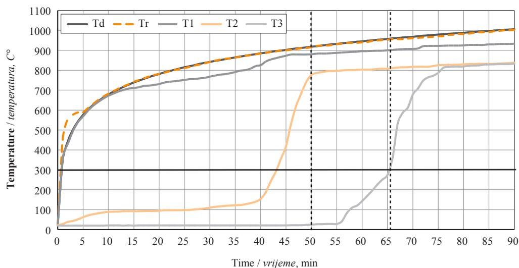
**Figure 6** Temperature trends of test specimen TS1 in thermocouples T1 to T3 depending on actually reached temperature  $T_r$  in fire furnace with marked significant time points,  $T_d$  is fire furnace reference temperature
