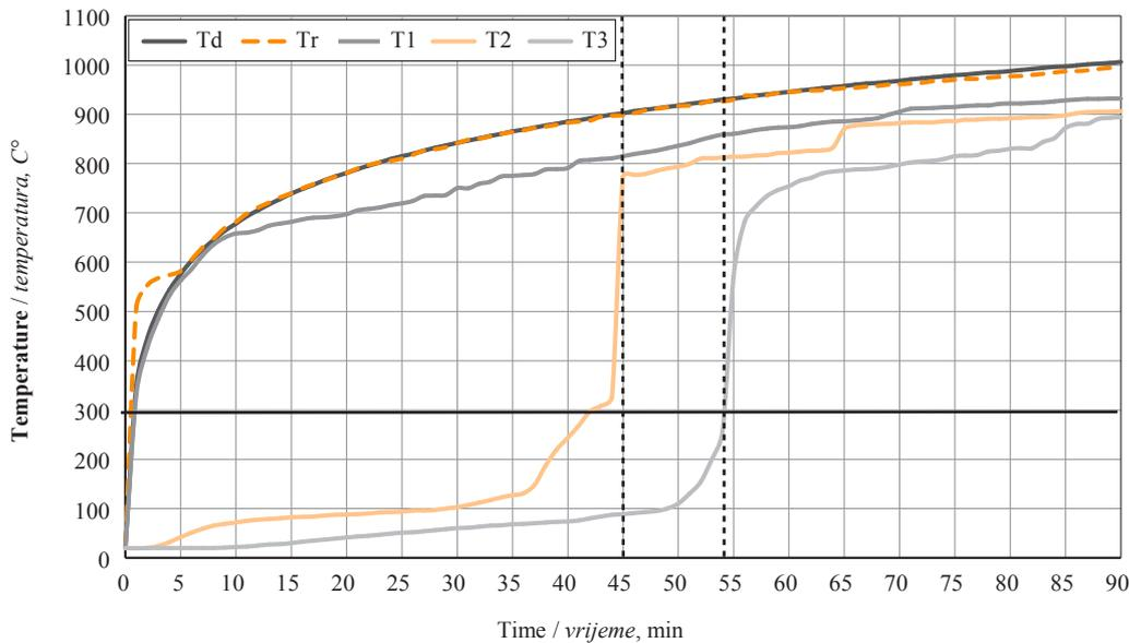
**Figure 7** Temperature trends of test specimen TS2 in thermocouples T1 to T3 depending on actually reached temperature  $T_r$  in fire furnace with marked significant time points,  $T_d$  is fire furnace reference temperature
