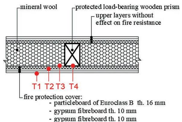
The test specimens were equipped with K-type thermocouples. The T1 thermocouples were placed on a heated surface. The T2 thermocouples were placed on gypsum-based board and the T3 thermocouples on wood-based board (oriented strand board or particleboard). The test specimens TS3 and TS4 still had T4 thermocouples in the joint under the wooden prisms.
