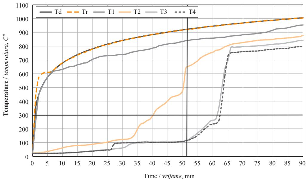
**Figure 9** Temperature trends of test specimen TS4 in thermocouples T1 to T3 depending on actually reached temperature  $T_r$  in fire furnace with marked significant time points,  $T_d$  is fire furnace reference temperature
