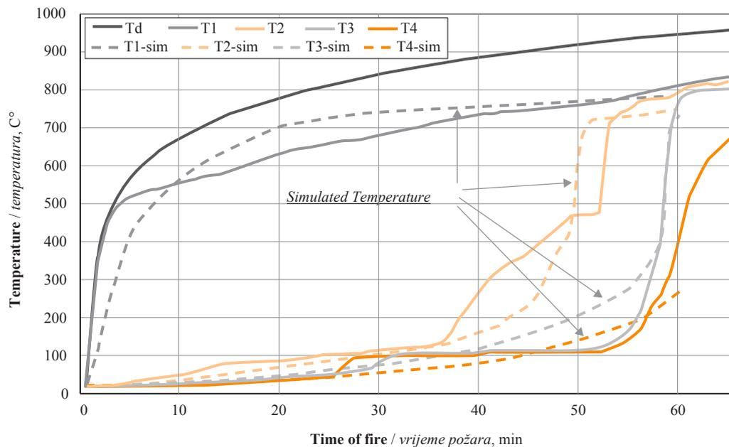
**Figure 10** Comparison of numerical analysis and fire test results of test specimen TS3, where  $T_d$  is fire furnace reference temperature, T1 to T4 are temperatures measured by thermocouples, T1-sim to T4-sim are temperatures obtained by numerical analysis
