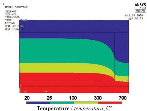
**Figure 11** Temperature distribution in cross-section in °C at the end of simulation (after 1 hour)
