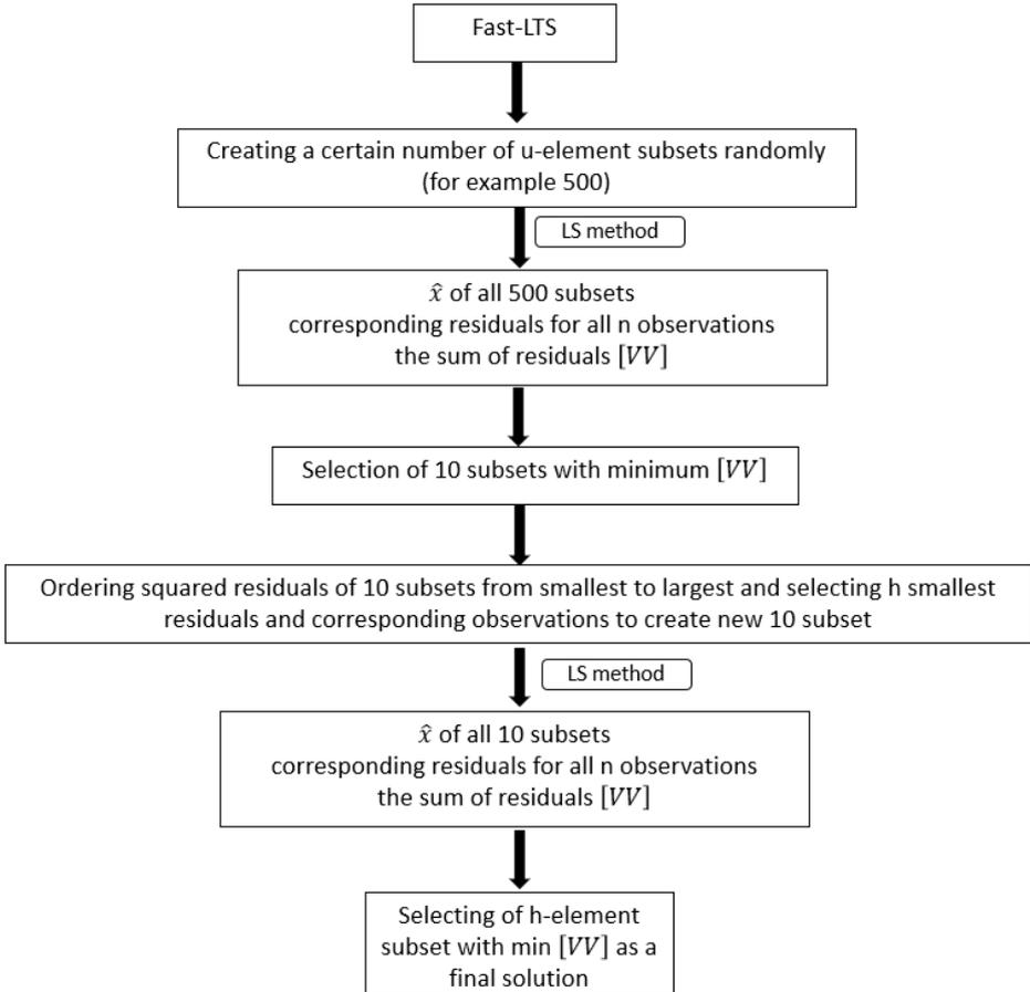
Fig. 3. The workflow of the Fast-LTS solution.
