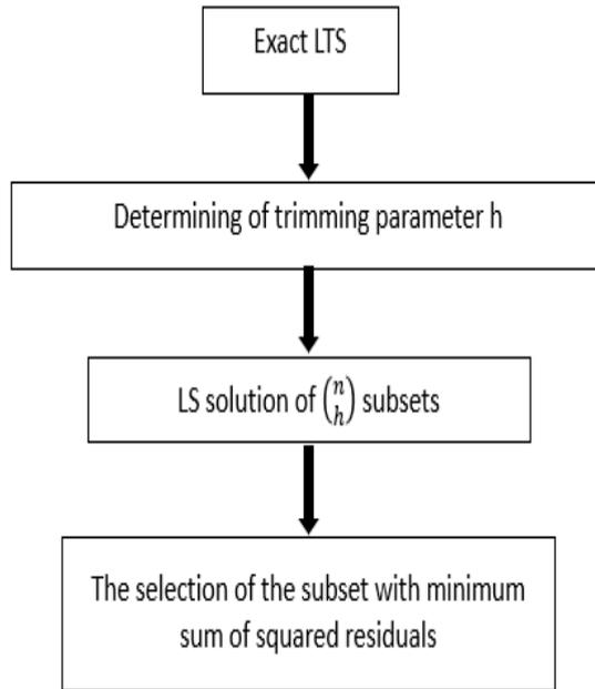
Fig. 2. *The workflow of exact LTS solution.*
