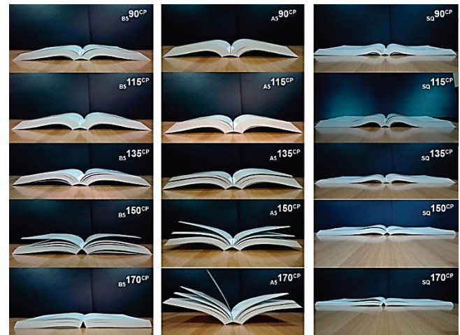
Figure 13 Perfect bound book appearance depends on a book format size (A5 format, B5 format, square format)
