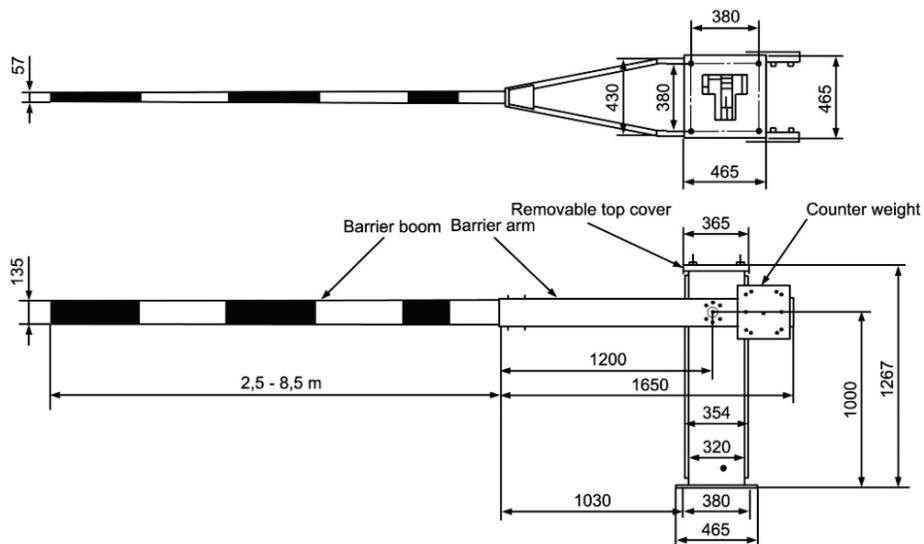
Figure 15 Top and side view of the PBH21 [31]
