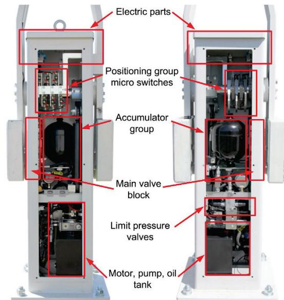
Figure 13 Barrier drive PBH21 modular architecture [31]
