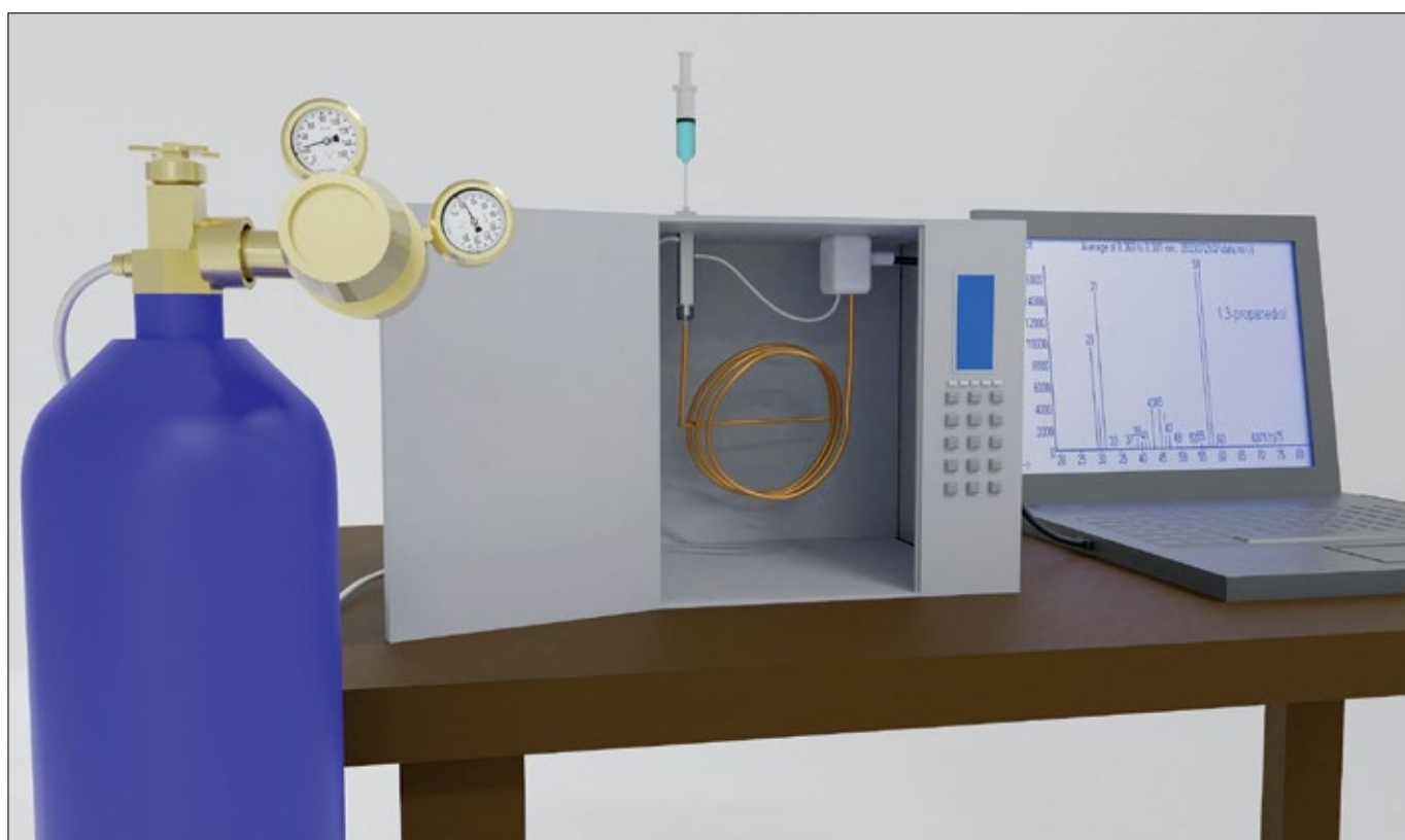
Figure 4. Illustration of main components of a classic gas chromatograph
