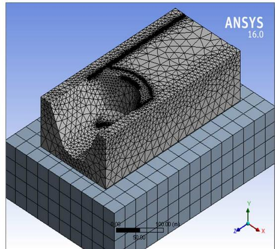
**Fig. 4** Model 3 Dam with soil and reservoir
