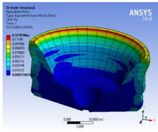
Fig. 5 Self-weight-induced deformation and stresses on a dam (without a soil foundation)
