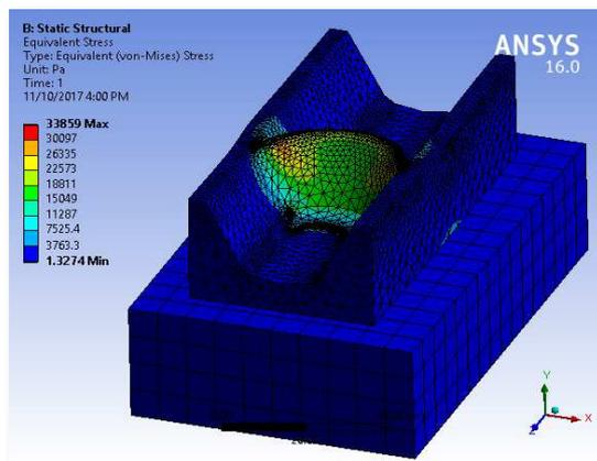
**Fig. 11** Results of simulating the effects of water pressures on the upstream and downstream sides of the arch dam
