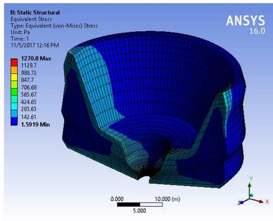
Fig. 13 Results of simulated uplift water pressure acting at the dam's bottom face
