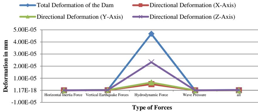
Fig. 22 Dam deformation due to various load cases
