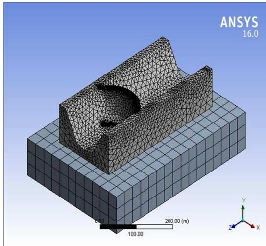
**Fig. 3** Model 2 Dam with soil foundation model
