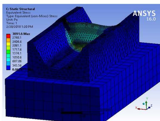
**Fig. 21** Results of simulated wave pressure, horizontal inertia forces, and hydrodynamics on the upstream face of the arch dam
