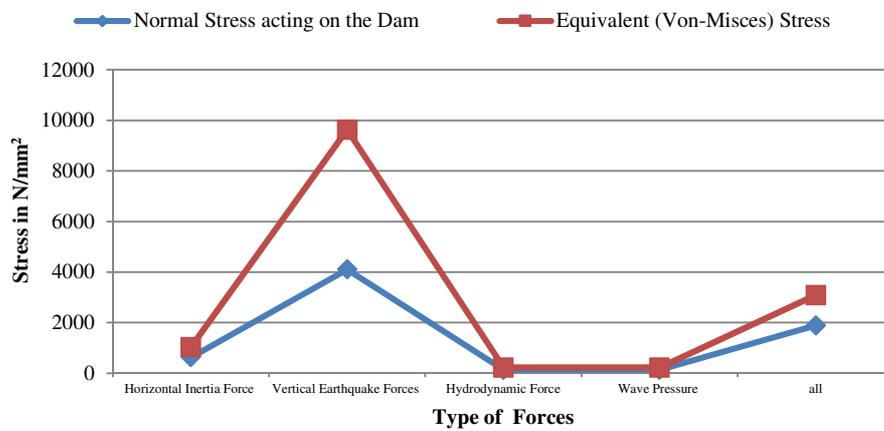
Fig. 23 Dam stress due to various load cases
