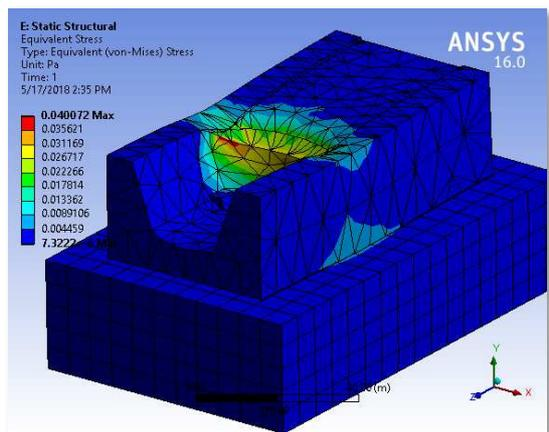
**Fig. 7** Deformation and stresses due to self-weight acting on a dam (soil foundation, reservoir)
