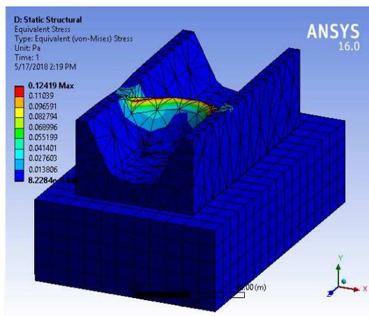
Fig. 6 Self-weight-induced deformation and stresses on a dam (with a soil foundation)
