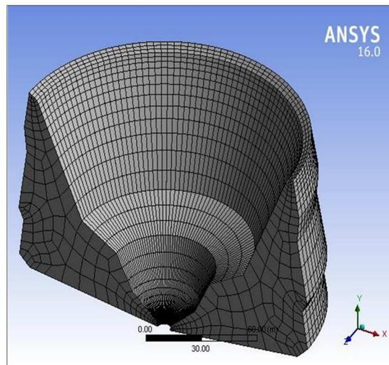
**Fig. 2** Model 1 Dam without soil foundation model
