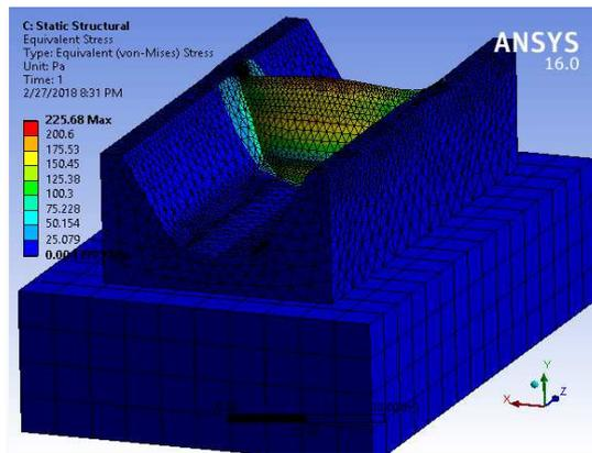
Fig. 17 Simulation of hydrodynamic forces occurring on the dam's upstream face
