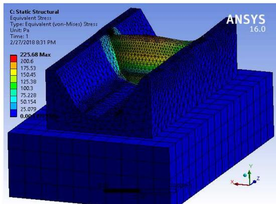
Fig. 20 Results of simulated vertical seismic forces occurring at the dam's bottom face
