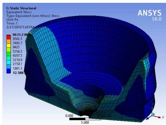
Fig. 19 Simulations of the effects of vertical earthquake stresses on the dam's bottom face
