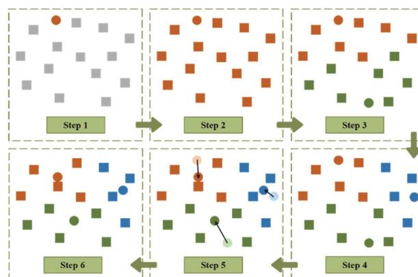
Figure 6 K-Means++ algorithm running step schematic diagram
