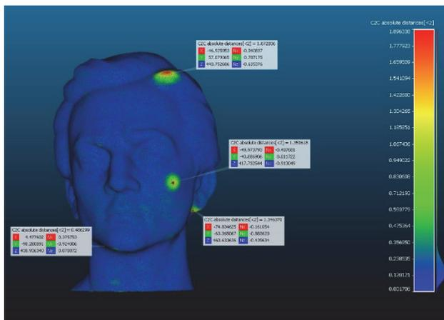
Figure 8 Results of the comparison of printed 3D models in CloudCompare software (OS1 and OSP1)
