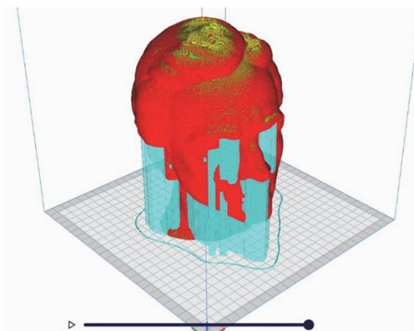
Figure 4 Preparing the 3D printing with UltiMakerCura software
