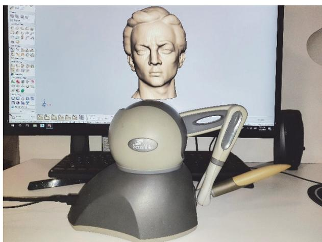
Figure 2 Phantom Omni haptic device used for adding local-inconspicuous bumps
