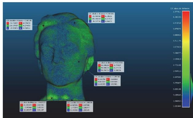
Figure 10 Results of the comparison of 3D models with built-in protection in CloudCompare software (virtual (OSP) and printed (OSP1))
