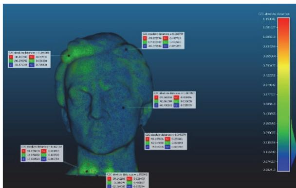
Figure 9 Results of the comparison of original 3D models in CloudCompare software (virtual (OS) and printed (OS1))
