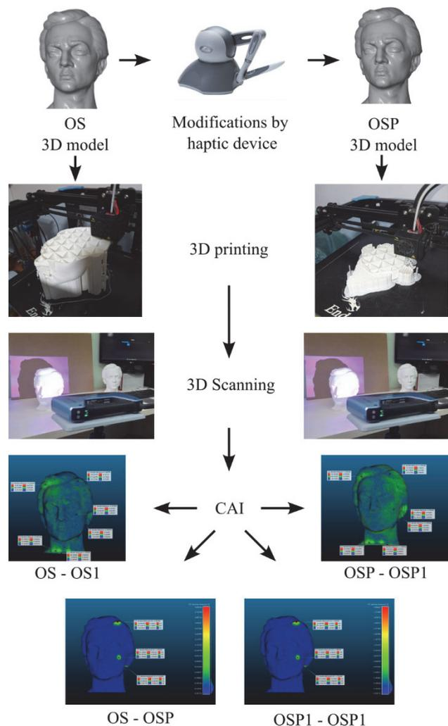
Figure 1 Proposed methodology of adding local, inconspicuous bumps on 3D digitized sculptures using a haptic device
