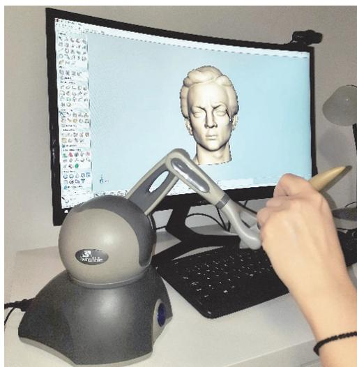
Figure 3 Sculpture modification in Geomagic Freeform software with the Phantom Omni haptic device
