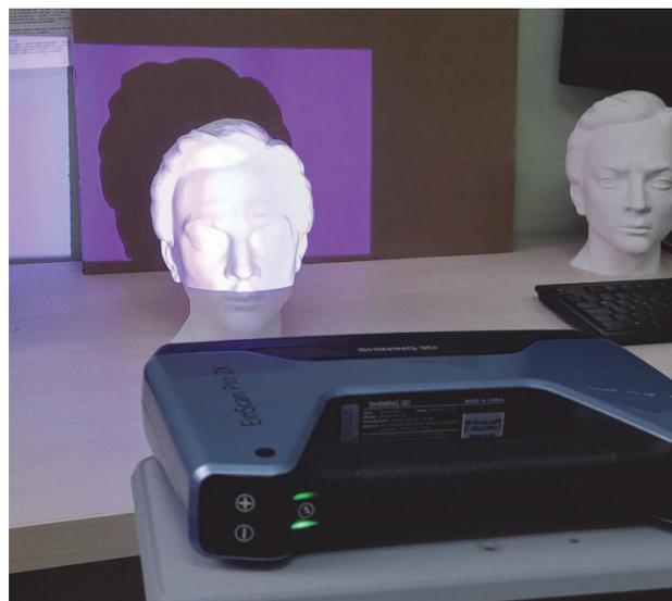
Figure 6 The process of 3D scanning in fixed mode using EinScan Pro 2X optical 3D scanner
