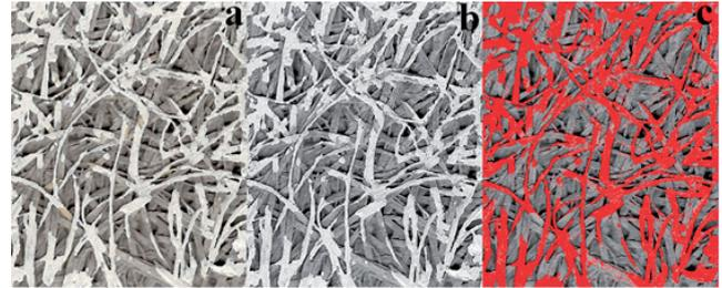
**Fig. 5.** Example of scanned image treatment in ImageJ. Colored and scanned composite board (a), scanned image transformed to 8 bit image (b) and processed image with already determined surface pixels (c).
