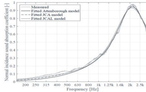
Fig. 3. Characteristic sound absorption coefficient for WWCB [7]
