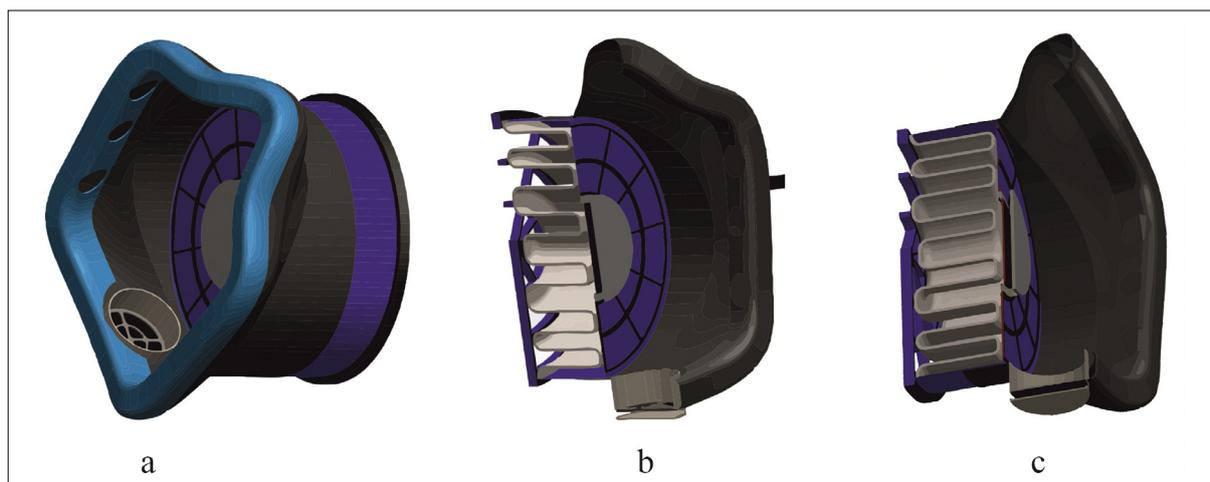
**Figure 3:** Suggested models for improving the design of the obturator filter respirator: a) with holes around the perimeter of the obturator; b) holes are made at the nasal bridge and cheeks; c) cutouts are made behind the perimeter of the obturator
