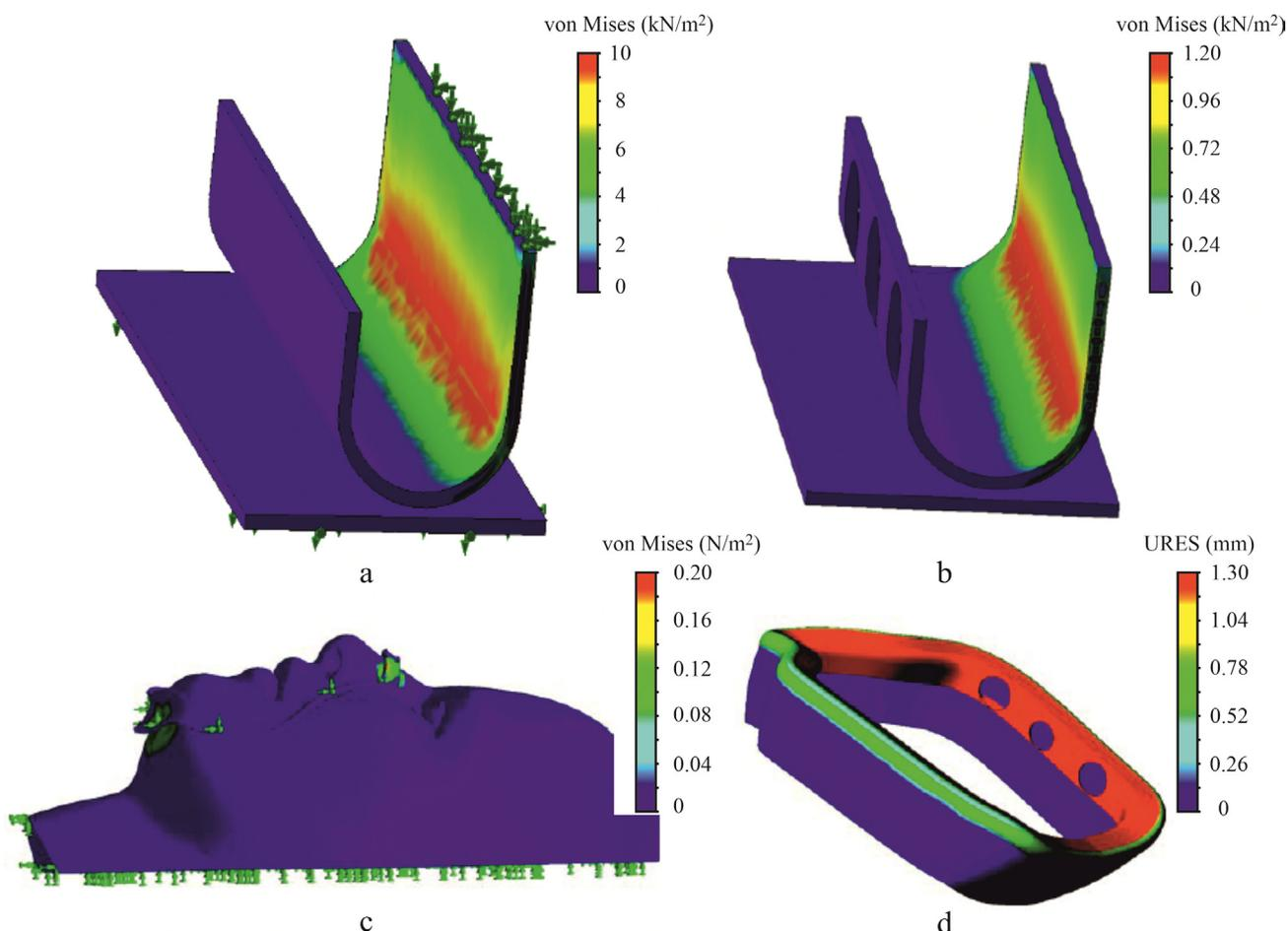
**Figure 8:** Distribution of forces along the obturation line of the filter respirator: non-perforated (a); perforated (b); on the calculation face model (c); on the calculation model of the respirator half-mask (d)
