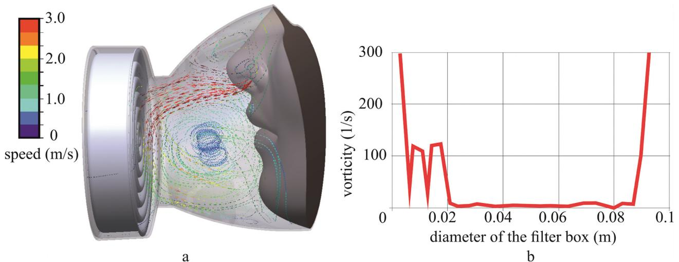
**Figure 6:** Interrelationship between flow vorticity and design parameters of a filtering half-mask: visualization of streamlines inside the half-mask when  $Q_s=30$  l/min,  $S_s=7$  mm<sup>2</sup>,  $k=9.55 \times 10^{-11}$  m<sup>2</sup> (a); dependence of the flow vorticity on the diameter of the filter box
