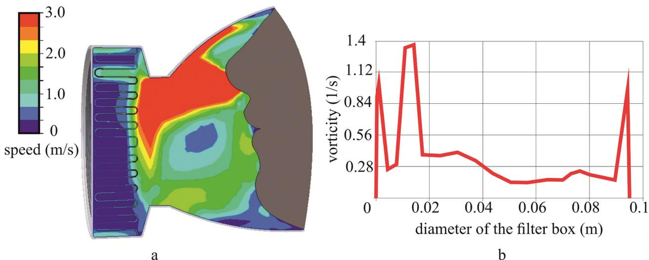
**Figure 7:** Interrelationship between airflow rate and filtering half-mask design parameters: visualization of airflow distribution inside the half-mask when  $Q_f=30$  l/min,  $S_s=7$  mm<sup>2</sup>,  $k=9.55 \times 10^{-11}$  m<sup>2</sup> (a); dependence of the air flow rate on the diameter of the filter box (b)
