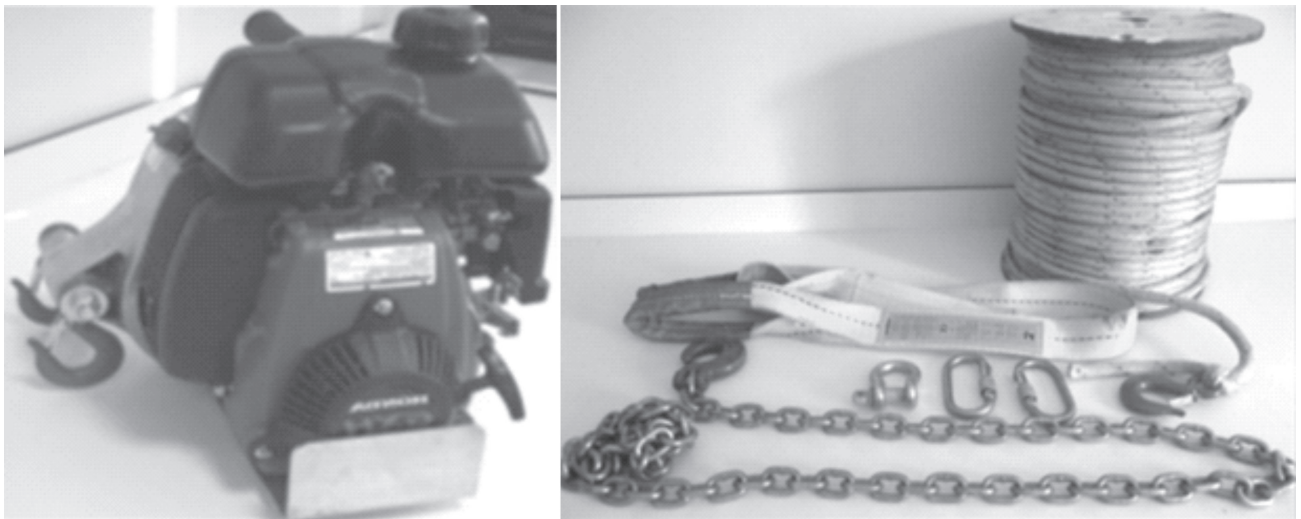
Fig. 3 Portable winch (left) and other equipment such as synthetic rope, polyester choker, metal locks, direction pulley and metal hooks (right) used in cable yarding operation
