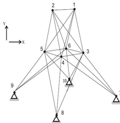
**Fig. 5** The structure of the 25-bar truss
