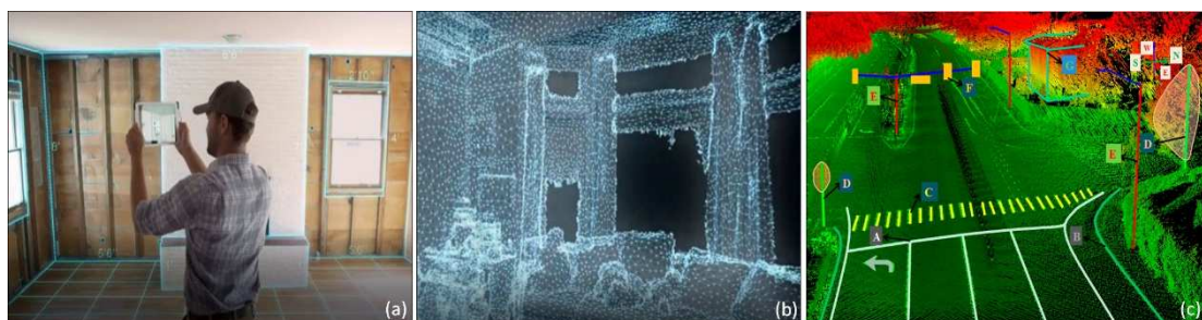
Fig. 14 Automatic spatial data capturing applications: a) Applications of special devices [103]; b), c) Application of 3D laser scanning [102]
