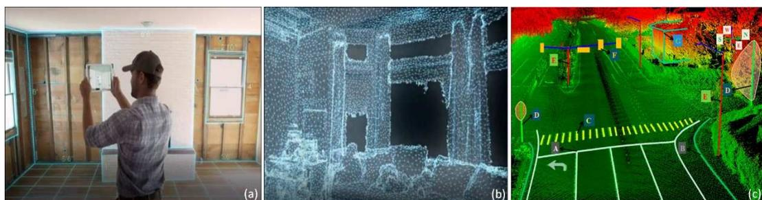
**Fig. 14** Automatic spatial data capturing applications: a) Applications of special devices [103]; b), c) Application of 3D laser scanning [102]
