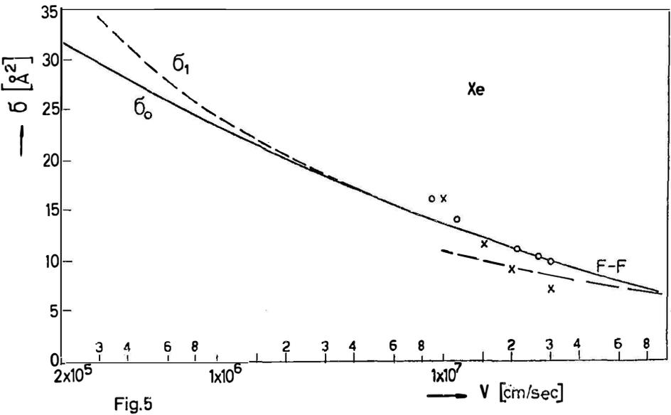
Fig. 1-5. Resonant double charge exchange cross sections. Curves  $\sigma_1$  and  $\sigma_0$  represent our calculations of the cross section with and without taking into account the direct interparticle interaction. Curves F-F and F-M are variational results of refs. <sup>10)</sup> and <sup>11)</sup>. Symbols  $\blacktriangle$ ,  $\circ$ ,  $\times$  represent the experimental data of refs. <sup>7)</sup>, <sup>8)</sup> and <sup>9)</sup> respectively.
