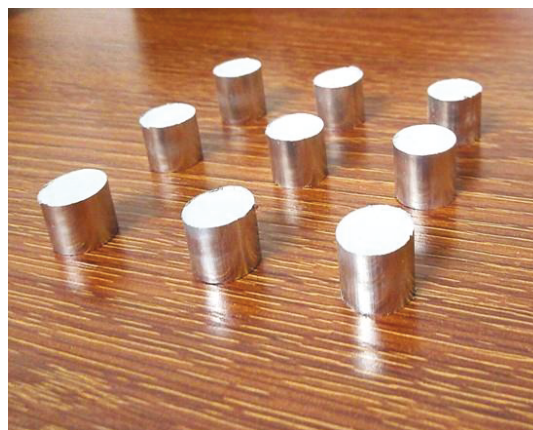
Figure 2. Sintered Al-10SiC and Al-20SiC composites
