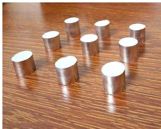
Figure 2. Sintered Al-10SiC and Al-20SiC composites
