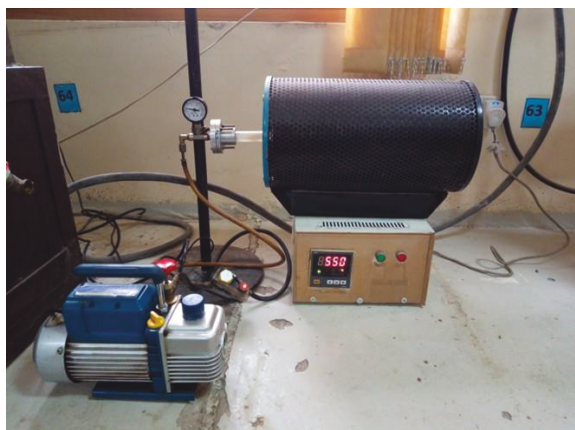
Figure 1. Vacuumed furnace system
