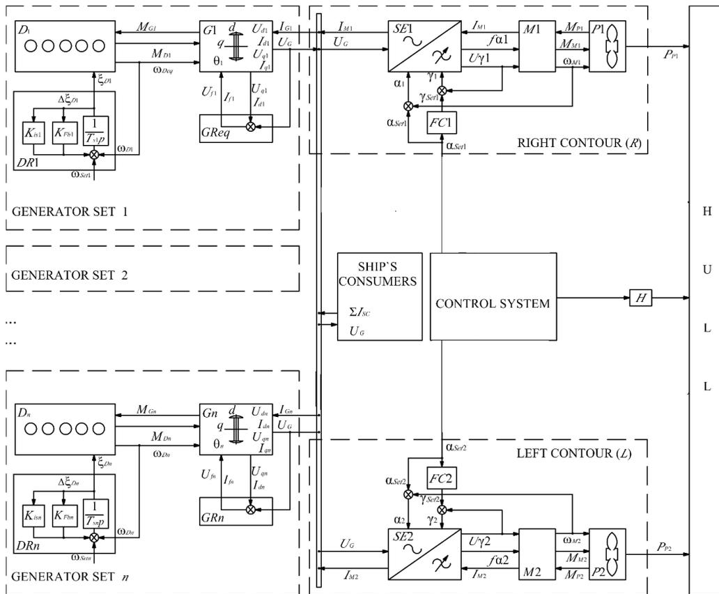
Figure 1 Structural diagram of the electric propulsion system
