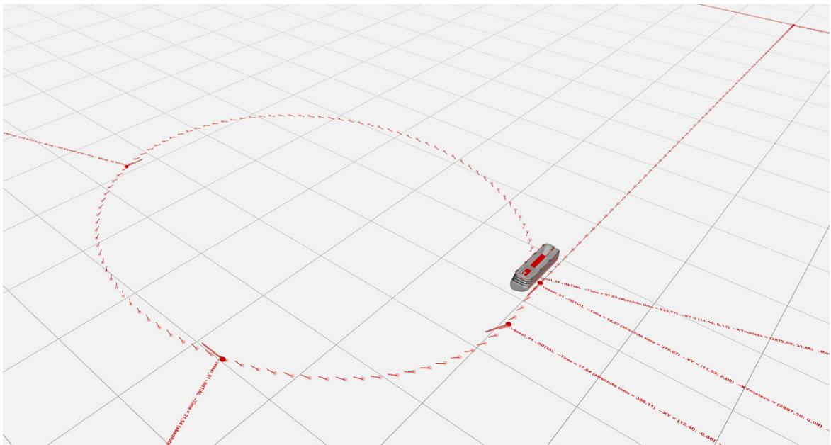
**Figure 3** Developed software screenshot with vessel trajectory when entering the turning circle maneuver with pivot points markers
