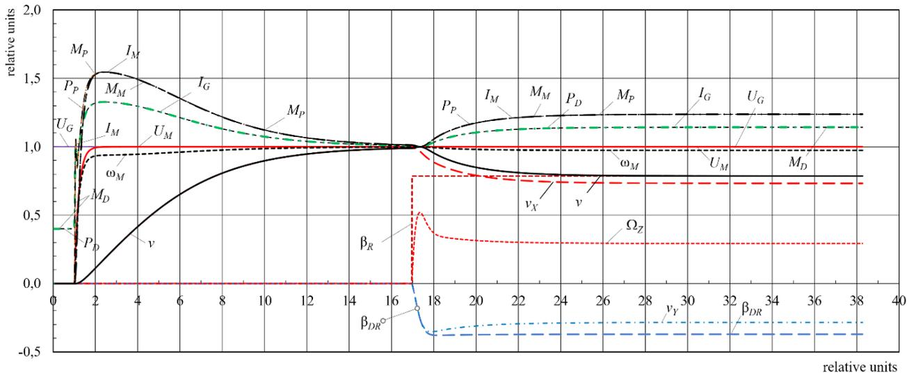
**Figure 2** The key indicators dynamics when performing “acceleration – enter to turning circle” maneuver
