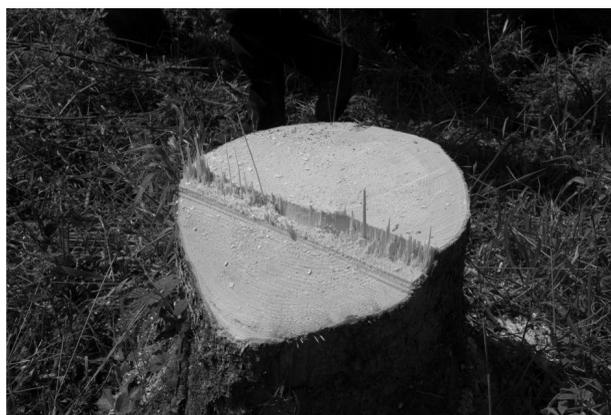
**Fig. 11** Stump as a result of field tests with felling head
