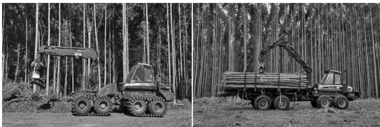
Fig. 1 Ponsse Bear harvester (left) and Ponsse Elephant forwarder (right) used in the study
