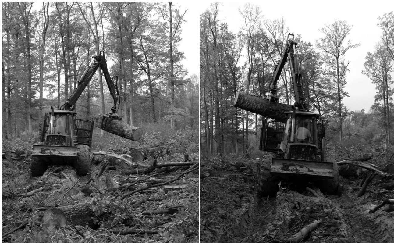
Fig. 4 Loading oak roundwood by a Timberjack 1710B
