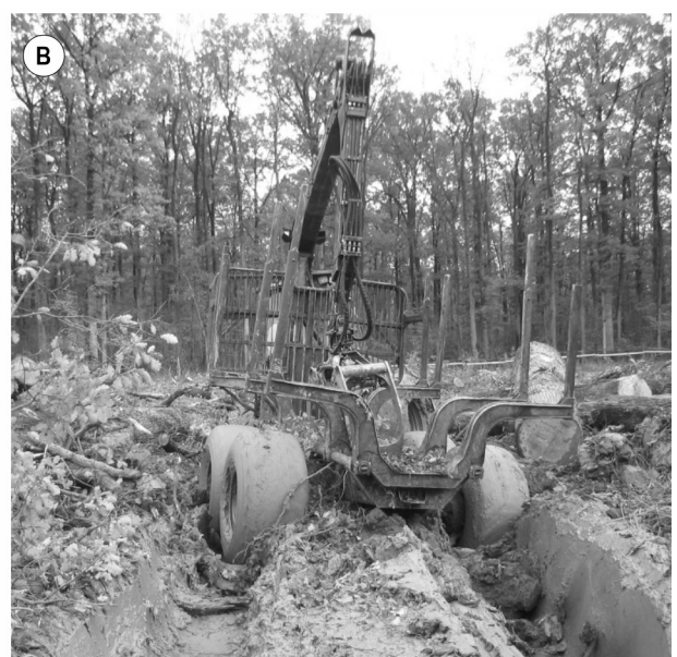
Fig. 7 Rutting A) median, 25%–75% confidence level and minimum-maximum each pass and B) unacceptable rut depth at study site
