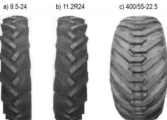
**Fig. 2** Overall view of tires tread patterns
