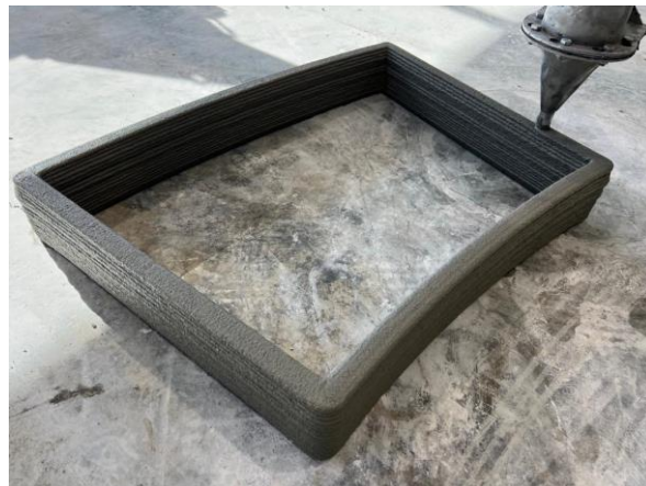
Figure 1. 3D printing with the mixture 008_CTM
