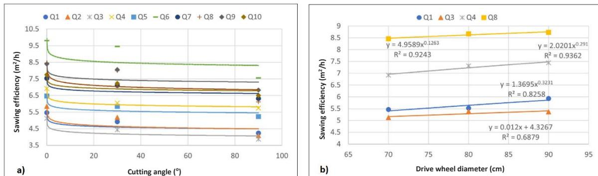
Figure 7 a) Influence of cutting angle on sawing efficiency b) Influence of drive wheel diameter on sawing efficiency, [6]
