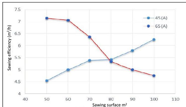
Figure 6. Influence of sawing surface and traction force on sawing efficiency, [2]
