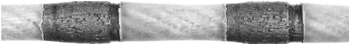
Figure 10. Wear of diamond beads due to excessive traction force, [22]
