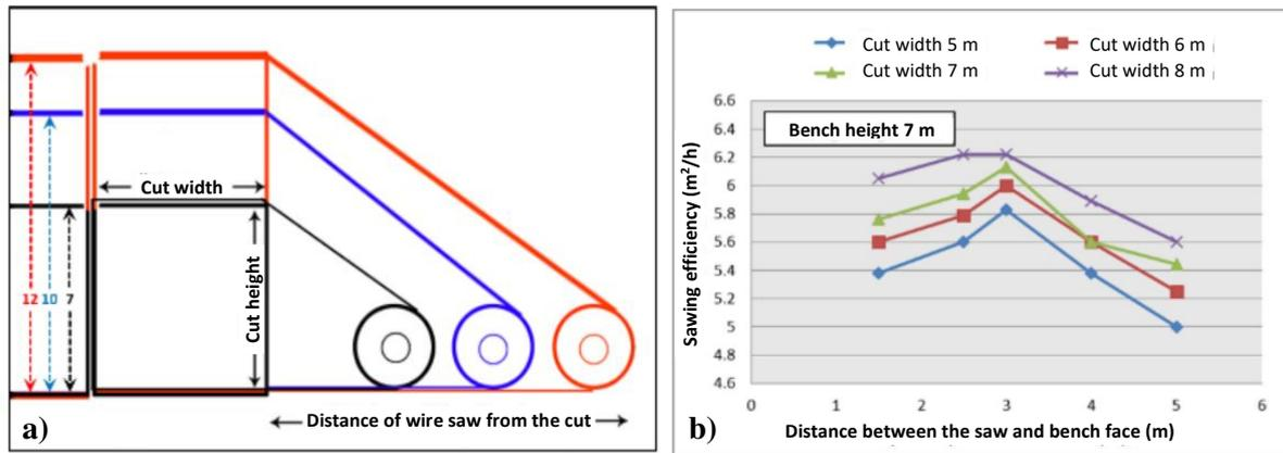
Figure 5. a) Geometry of the vertical cut depending on the position of the diamond wire saw
