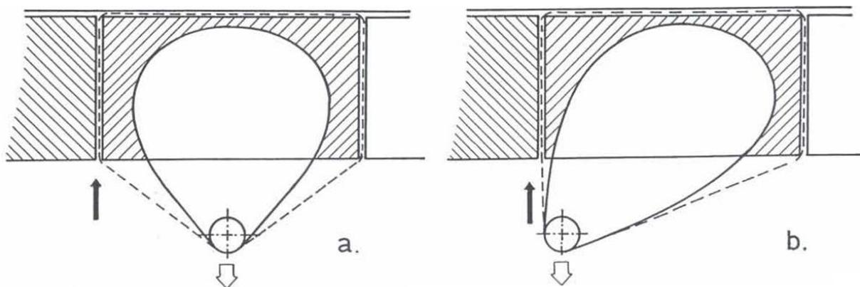
Figure 4. Possible positions for a horizontal cut, a) central position, b) lateral position of the saw, [1]
