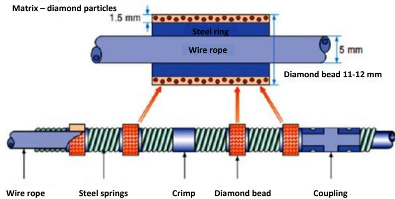
Figure 2. Diamond wire structure, [4]
