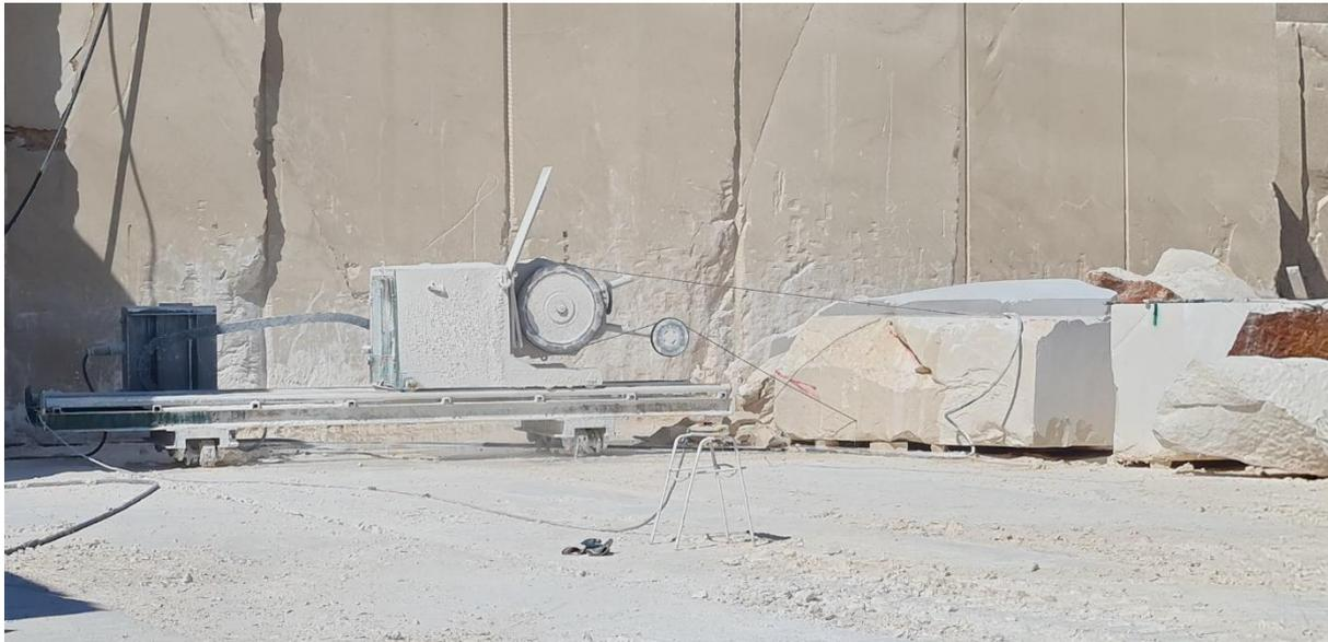
Figure 1. Diamond wire saw and control unit
