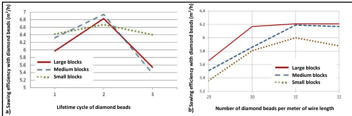
Figure 9 a) the influence of the life cycle of diamond beads on the sawing efficiency b) the influence of the number of beads on the sawing efficiency, [19]
