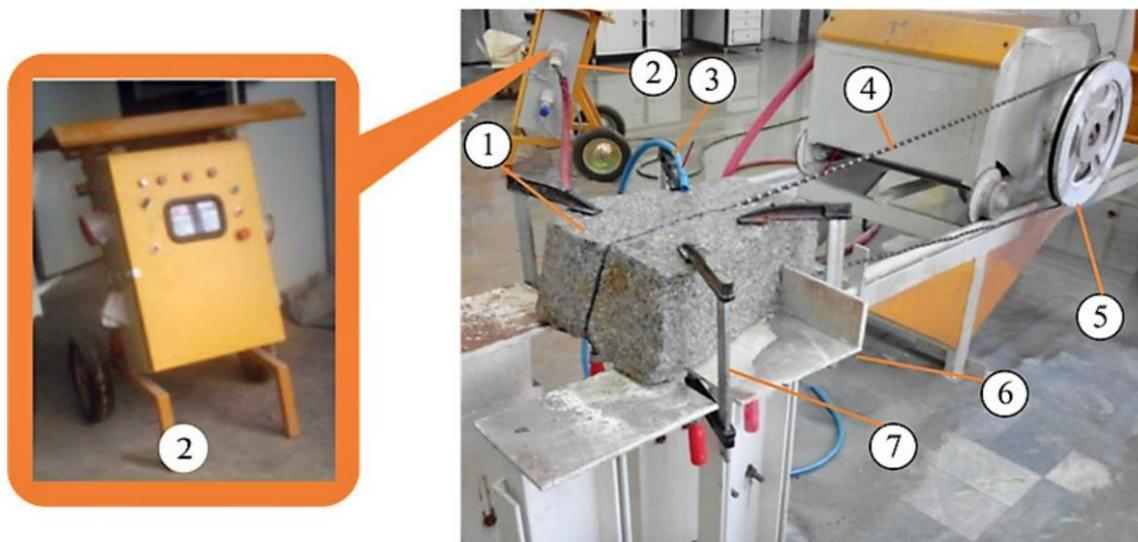
Figure 3. Laboratory diamond wire saw: 1 - Rock sample; 2 - Energy consumption measurement unit; 3 – Inflow of cooling water; 4 - Diamond wire; 5 - Drive wheel; 6 - Platform; 7 - Clamps for samples, [13]
