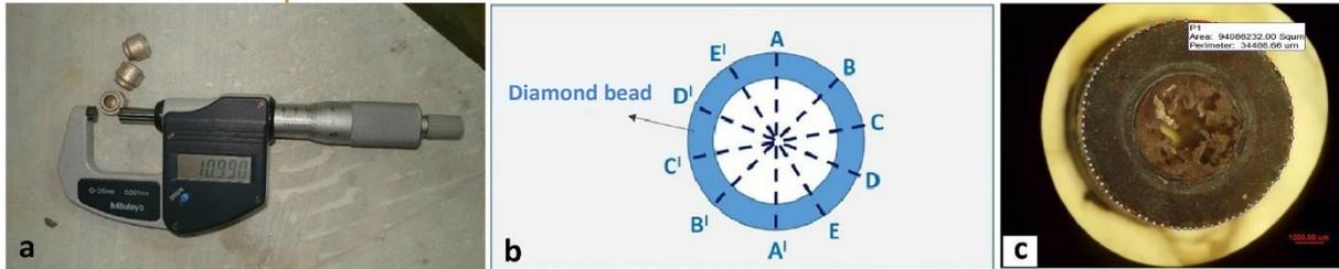
Figure 8. a) micrometer b) bead diameter measurement position c) microscopic image of a bead, [17], [18]
