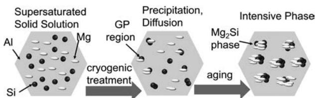
Figure 6 Intensive precipitates principle
