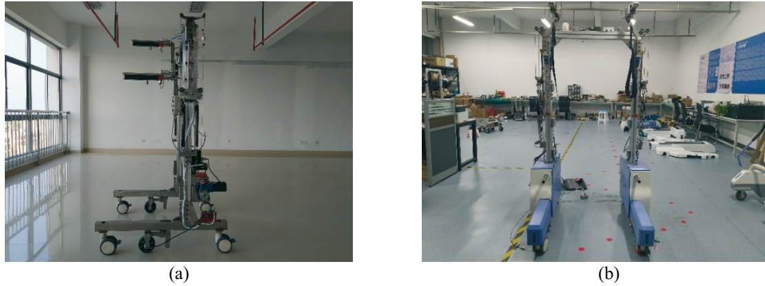
Fig. 13 Experimental platform for testing the steering error of the rehabilitation robot
