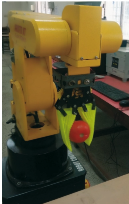
Fig. 6 Developed gripper attached to an industrial robot
