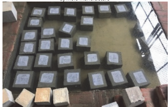
b) Curing concrete specimens in water
