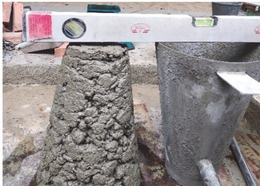
Figure 6 Measuring concrete slump
