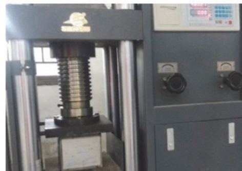
Figure 8 Compression of specimens for determining compressive strength of concrete
