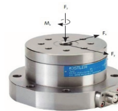
Figure 3 The used dynamometer in tests and measuring ranges [22]
