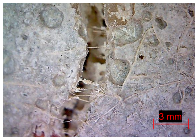
Figure 10. Bridging behaviour of jute fibre
