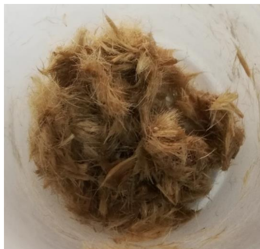
Figure 5. The appearance of jute fibres impregnated with bacterial spores
